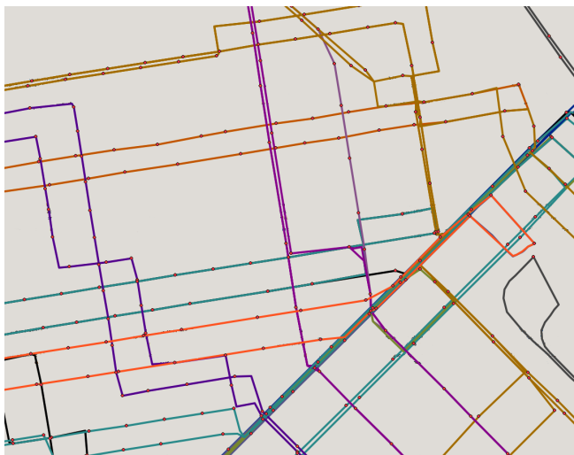
Figure 2: Example transit network structure built from open transit data with no link travel times defined.
